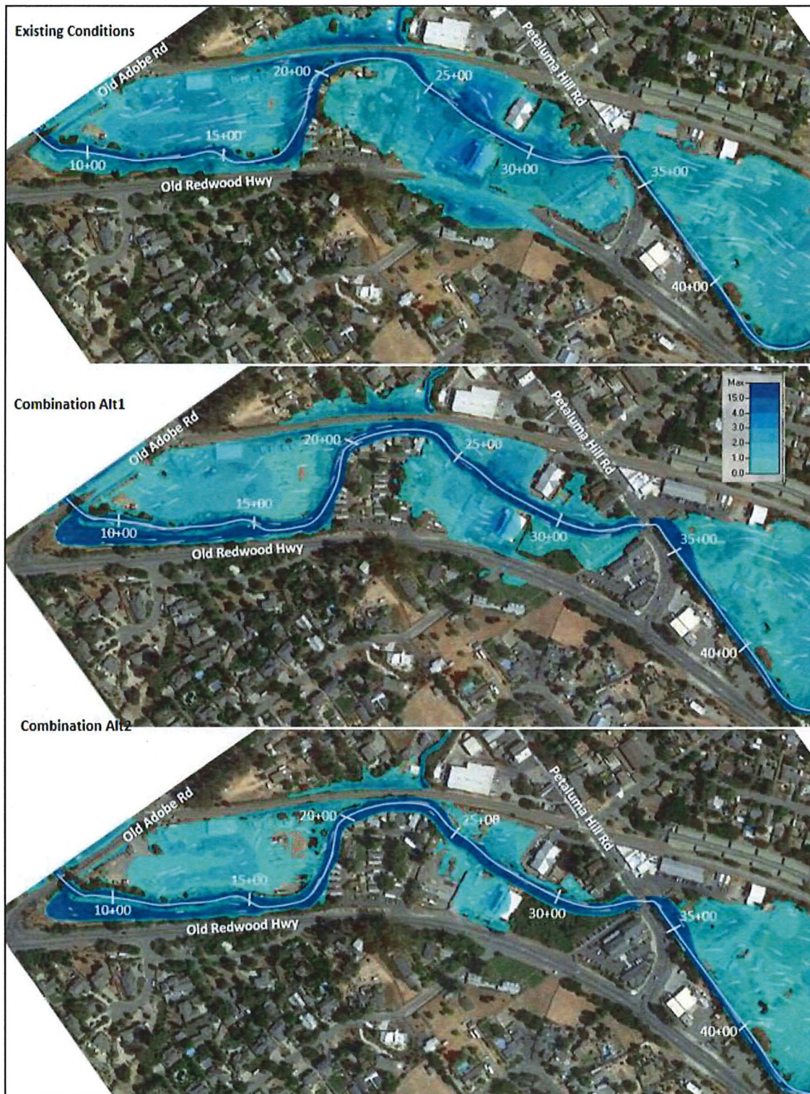
Figure 38. Water depths and flooding extents during the 10-yr storm for Existing Conditions and the two Combined Alternatives in downtown Penngrove.
