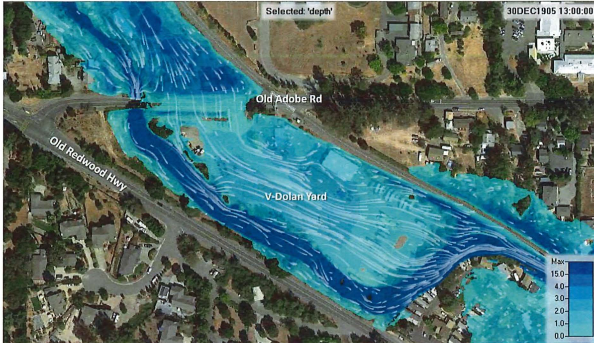
Figure 14. Existing condition predicted flood depths and extent during the FEMA 10-yr storm peak from Old Adobe Road through the V-Dolan yard.
