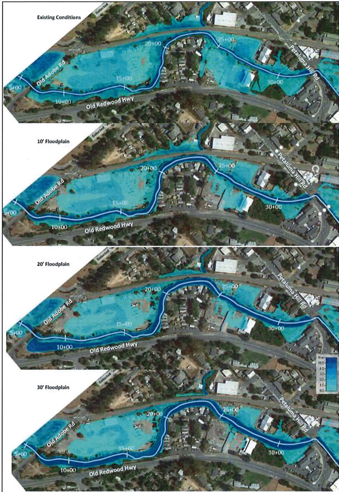
Figure 28. Simulated water depths during the 12/15/16 (Calibration) flood event under existing conditions (top) and the three floodplain bench alternatives (bottom three).
